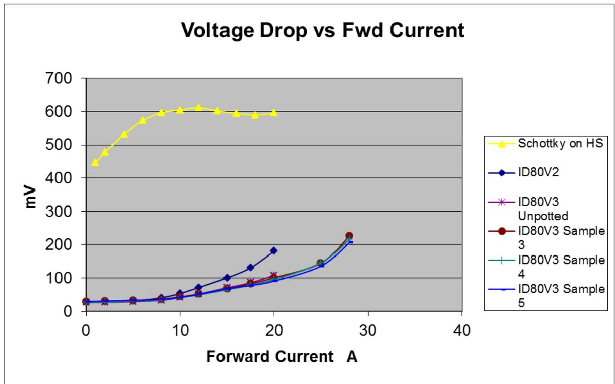
The voltage drop is measured from terminal to terminal of the module.
