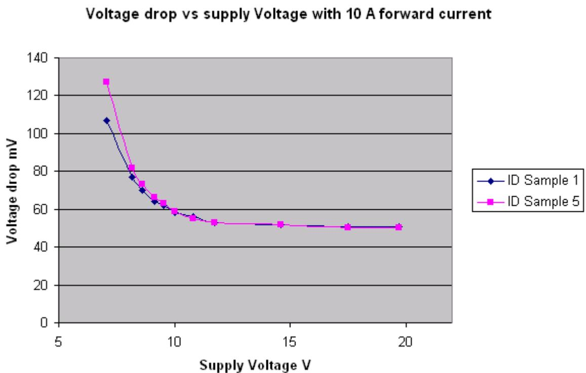
The minimum recommended supply voltage is 9 V. The maximum is 90 V. The module is suitable for battery systems with nominal system voltages from 12 to 72 V.
