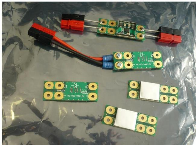
Dual terminals are provided for the Anode and for Ground at the Anode end. This is to facilitate fitting to busbars. It is possible to stack the modules side by side and run parallel busbars for Anode/Ground/Cathode as required.
