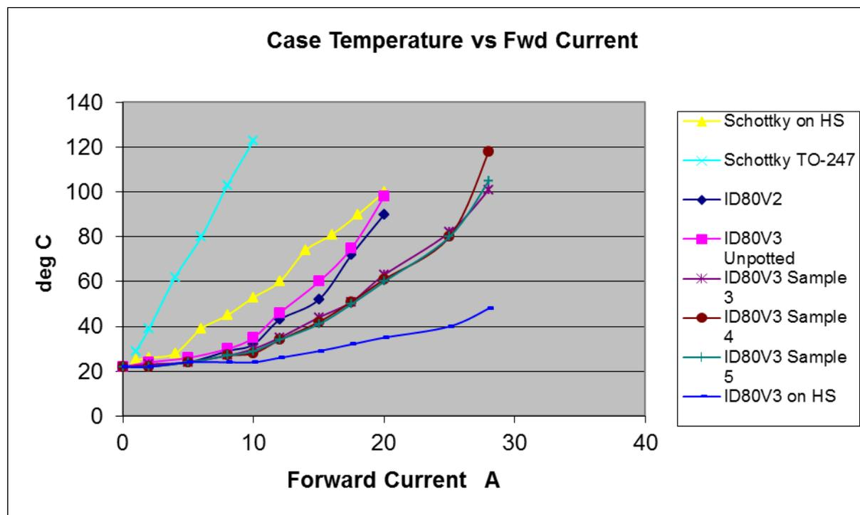
Again, a Schottky diode with and without heatsinking is included for comparison, as is the earlier ID80V2.
